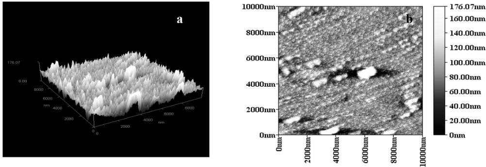
Fig: 4: Surface morphology of  $\text{Ag}_2\text{O}_3/\text{Ps}$  oxidized at 623K a- (3D), b- (2D).
