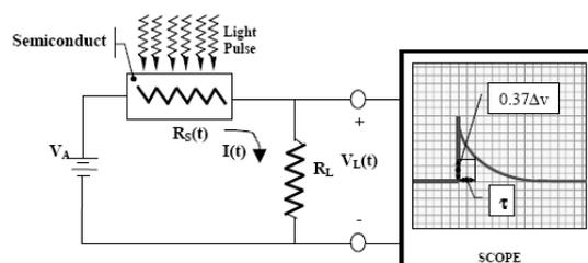
Fig. 1: Experimental setup for carrier life time measurement.
