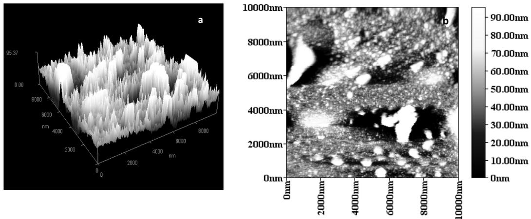
Fig. 3: Surface morphology of as deposited silver thin film (Ag) /Ps a- (3D), b- (2D).
