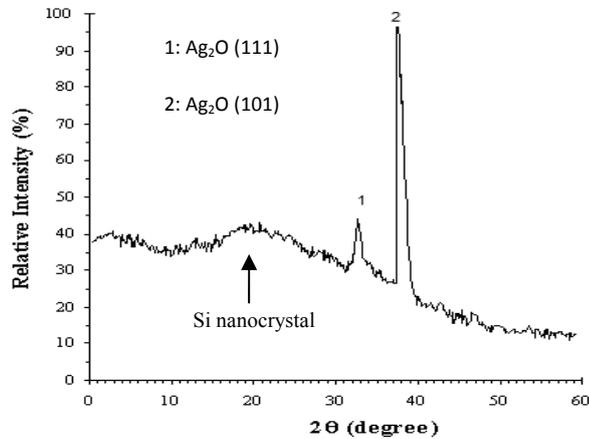
Fig. 2:  $\text{Ag}_2\text{O}_3/\text{Ps}$  a-x-ray diffraction pattern.
